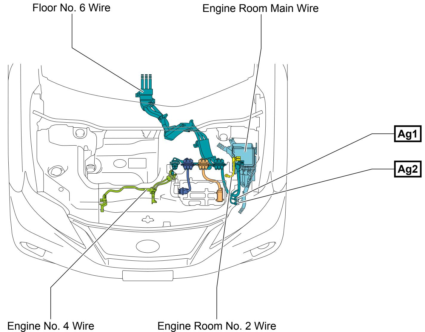
Wire and Wire in Engine Compartment <LHD>
